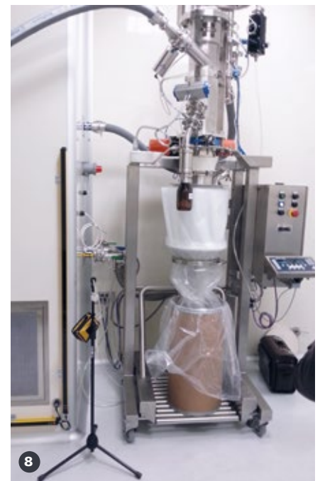
8: Small bin filling station with continuous liner filling head
