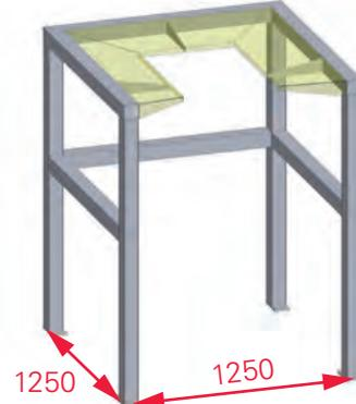
Fig.: Table frame with FIBC support
