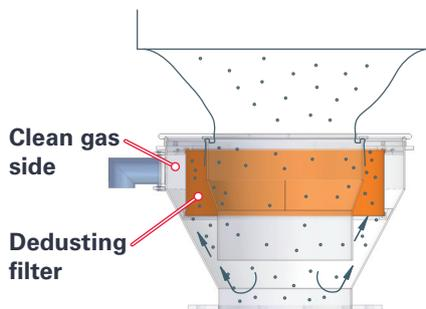
The integrated dedusting filter makes sure that dusty and dust-free air (clean gas side) are separated, preventing product from getting to the clean gas side or into the extraction.
