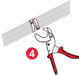
4 Position the liner scissors between the two clips and separate the liner bundle with a single cut.
