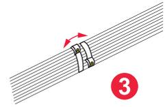
3 A second cable tie is positioned close to the first one, twisted against each other, and fixed in the same way.
