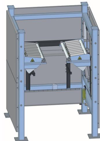
**Description:** FIBC support with agitation unit as discharge aid
