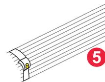
5 The short excess end remaining at the two ends of the liner bundles is safely closed by the liner clip.
