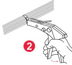
2 By actuating the closing tool, the liner clip is tightened, the free end cut off and the closure head locked.
