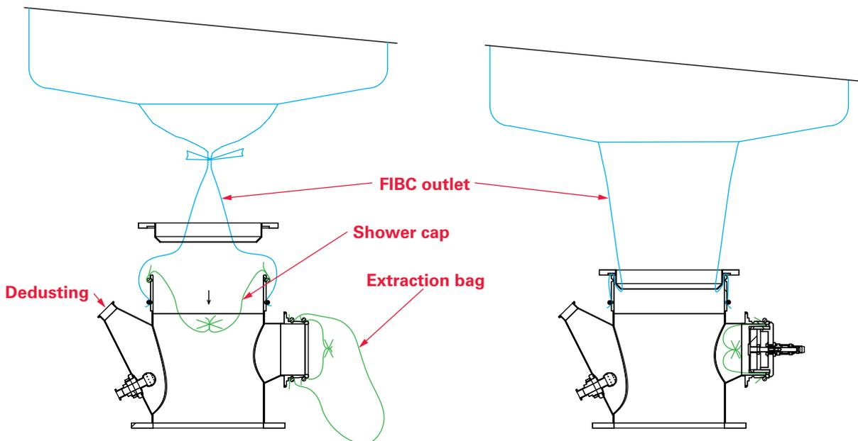
The FIBC outlet is fastened to the product tube using the connection ring.
