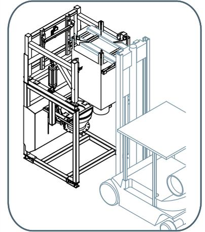
**Forklift as lifting device hangs the FIBC into the modular frame**
