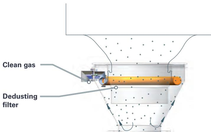
Dust is deposited in the connection system at a dedusting filter with pneumatic cleaning and thus remains inside the system without loss.
