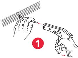
1 Place a liner clip around the liner bundle, pull it tight by hand and insert its end into the closing tool.
