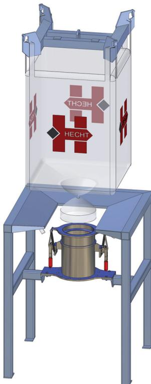
The compact connection system distinguishes itself by its easy handling. For discharging, you just have to pull the closed FIBC outlet over the product tube and fix it using the sealing flange. The latter is possible using the **two-hand lever mechanism**, which makes sure that the operator cannot squeeze his/her fingers between the sealing flange and the product tube in case of proper handling. Then, the FIBC outlet can be opened and the FIBC can be discharged in low-dust mode.
