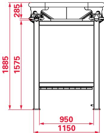
The combination with an individually selected connecting system and an outlet tensioning device make the SAT-VB a tailor-made big bag discharge station for your process. There are numerous options- ranging from a mechanical tensioning device with outlet connecting system (AAS) to a pneumatic tensioning device with liner connecting system "Easy Connect" (LAS-EC).
